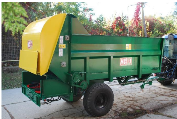
Fig. 10. Manure spreading machine for orchards, operating in strips near the tree trunks (MGL-3)
